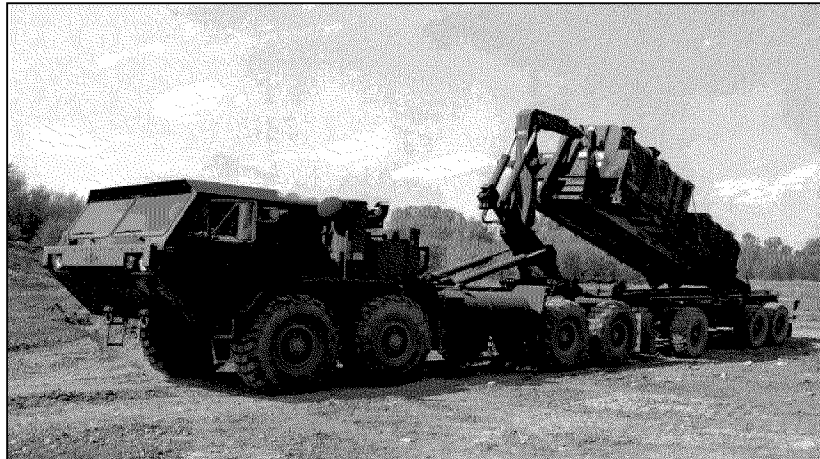
Figure 9. The Heavy Expandable Mobility Tactical Truck with Load Handling System (HEMTT-LHS)
